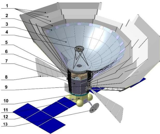
Fig. 1. Millimetron space observatory concept. 1 - Sun shields; 2 - Cryo-shield; 3 - Primary mirror's petal; 4 - Secondary mirror; 5 - Central part of Primary mirror; 6 - Cryo-container; 7 - Heat exchanger (radiator); 8 - Warm container; 9 - Sunshields supporting truss; 10 - Adapter ring; 11 - Service module; 12 - Solar power array; 13 - High gain antenna.
