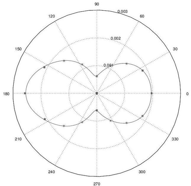
Fig. 2. Approximation of resultant force of light radiation pressure upon Millimetron depending on rotation angle in the radiator's plane (solid line) and results of Monte-Carlo simulation (dots), Newtons.
