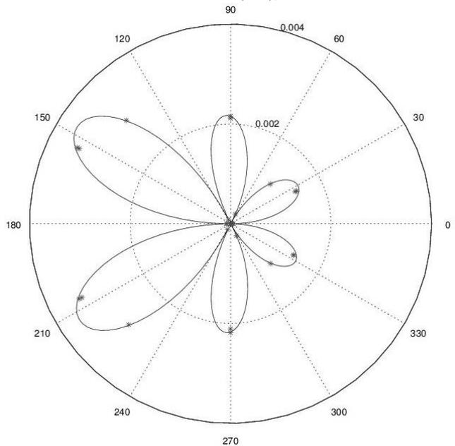
Fig. 3. Approximation of resultant moment of light radiation pressure upon Millimetron depending on rotation angle in the radiator's plane (solid line) and results of Monte-Carlo simulation (dots), Newtons x meters.
