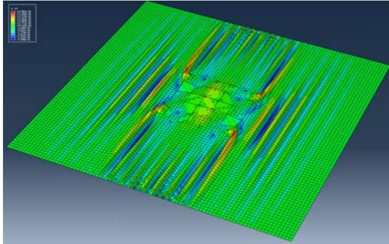
Fig.1 An example of FEM analysis of a membrane with a small thin film with different stiffness
